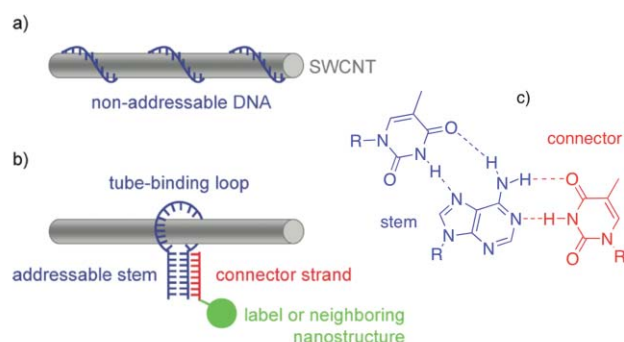
Fig. 12 SWCNT complexed with DNA (a) single-stranded oligonucleotide helically wrapped around a nanotube, (b) hairpin DNA (blue) binding both to a SWCNT and a complementary third strand (connector, red), (c) T-AT triplet (Reprinted with permission from ref. 119. Copyright 2010 American Chemical Society).
